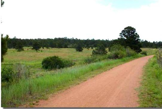
**Tier 1**, Trail, 8-foot wide average compacted crush limestone trail surface with shoulders
