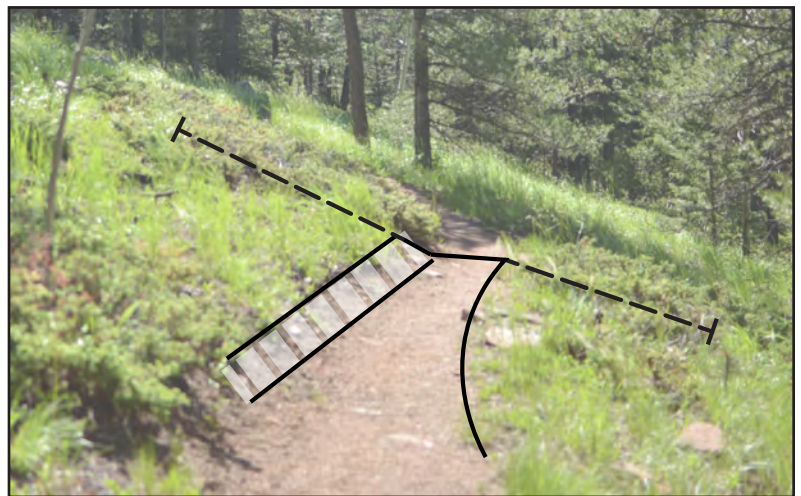
EXAMPLE OF PROPER TRAIL OUTSLOPE
