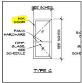
Please clarify if door no. 134A and 134B are intended as storefront doors (anodized aluminum) or hollow metal with a full glass panel.
