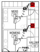
We assume these switches and switch leg need removal for new scope shown on E-L-101.N (new occupancy sensors) and the lighting is to remain as is. Please confirm and clarify if otherwise.
