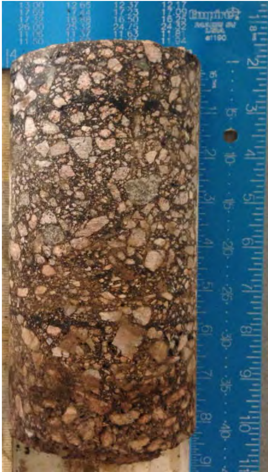
Pavement Core at SW-P-06 Westbound lane, 8 inches thickness measured
