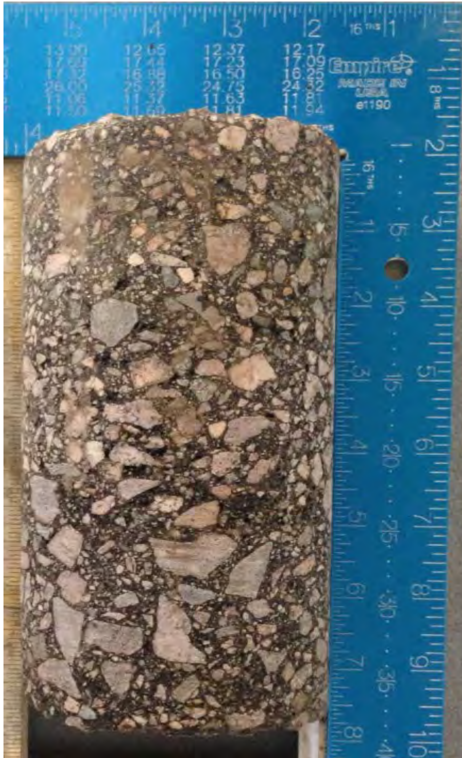
Pavement Core at SW-P-03 Eastbound lane, 7.5 inches thickness measured
